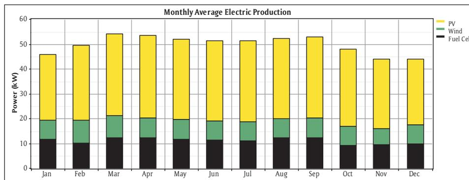
Figure 10: Monthly production of electricity for optimized system-II.
