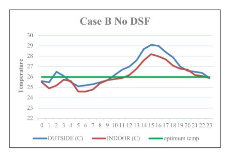
Figure 10 Hourly temp conditions without DSF.
