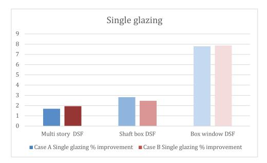
Figure 20 DSF performance in case A and B using single glazing.
