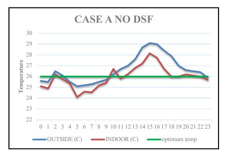
Figure 9 Hourly temp conditions without DSF.
