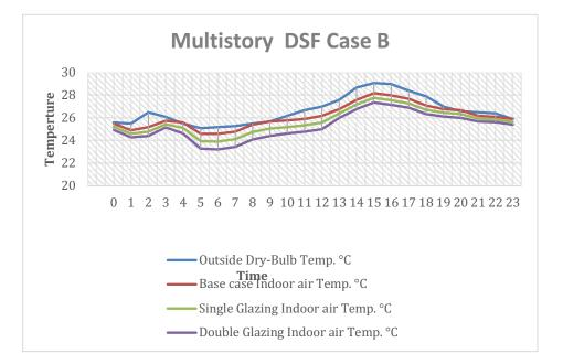
Figure 13 Hourly temp conditions with multi-story DSF.
