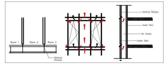
Figure 14 Floor, elevation and section of Shaft box (drawn by author).
