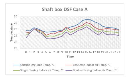
Figure 15 Hourly temperature conditions with Shaft box DSF.
