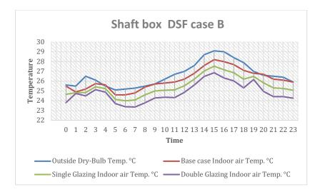
Figure 16 Hourly temperature conditions after integrating with Shaft box DSF.
