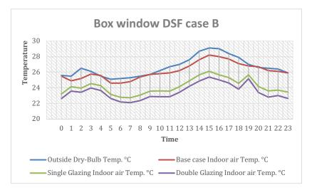
Figure 19 Hourly temp conditions with Box window DSF.
