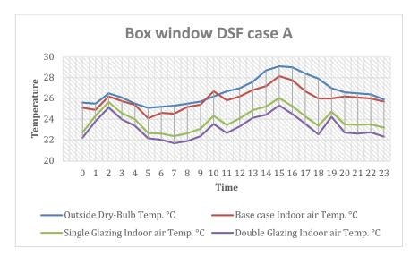
Figure 18 Hourly temp conditions with Box window DSF.
