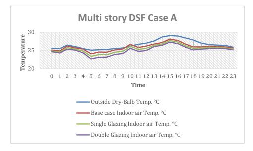
Figure 12 Hourly temp conditions with multi-story DSF.
