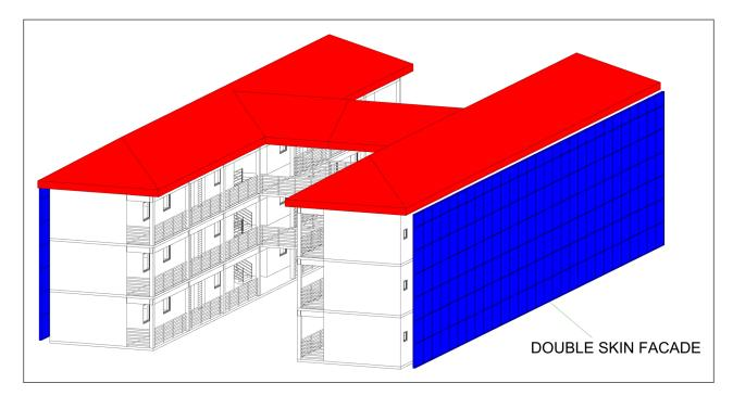
Figure 5 Case A showing the façade of the building with DSF attached.
