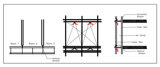
Figure 17 Floor, elevation and section of Box window (drawn by author).
