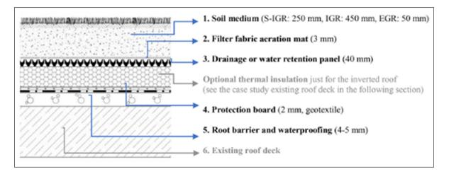
Figure 25 Layers of green roof used in the simulation (Motlagh et al., 2021).
