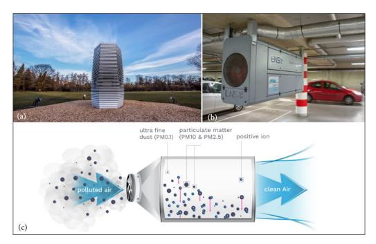
Figure 7 (a) The ENS systems outdoor application. (b) Aufero's device installed in a car parking. (c) A diagram for the positive ionization technique of ENS air purification technology (Environmental Nano Solutions, 2016).
