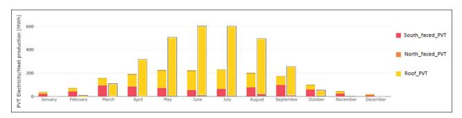
**Figure 8** Overview of the PVT production, the left column in every month is the electricity [MWh] production and the right is heat production [MWh].
