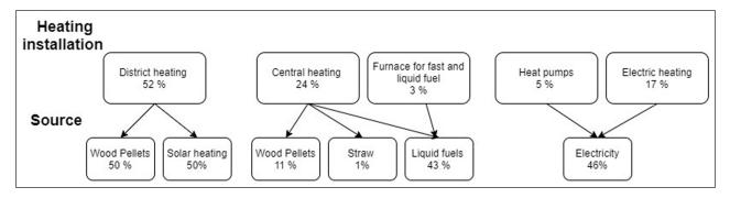
Figure 5 Different heating installation and sources provided by the BBR register.
