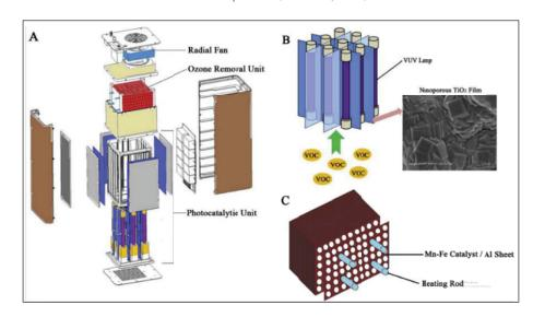
Figure 1 Diagram of the VUV-PCO air purifier (A), the photocatalytic unit (B) and the ozone removal unit (C). (Xu et al, 2018).
