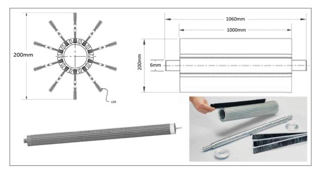
Figure 9 Dimensions and design of the hub.
