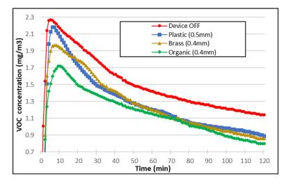
Figure 16 Monitoring results of VOC concentration.
