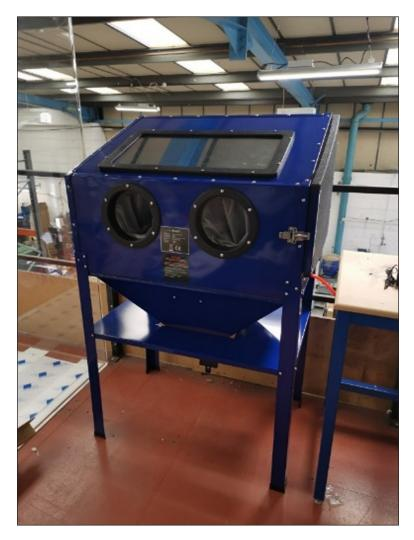
Figure 3 MAXBLAST Heavy duty sand blasting chamber 220 L.
