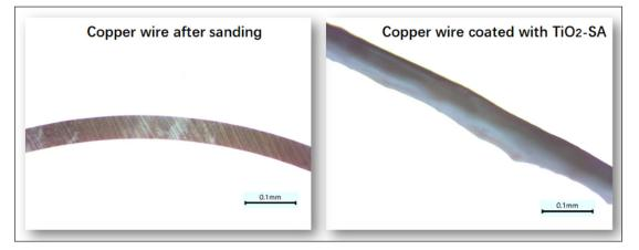
Figure 7 Microstructure of the copper wire with and without coating.
