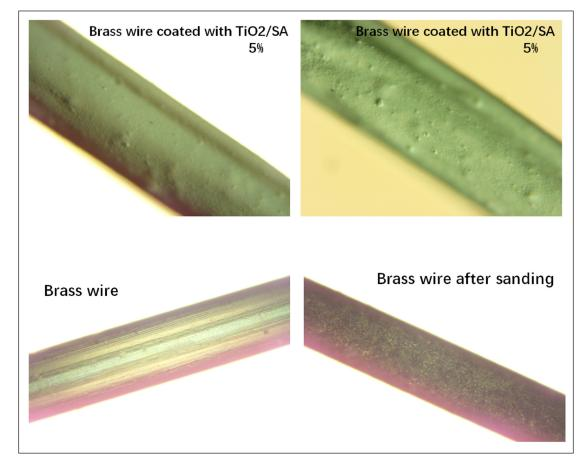
Figure 8 Microstructure of the brass wire with and without coating.
