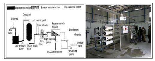
Figure 5: Schematic diagram for fully automated Containerized Skid Mounted Packaged RO Brackish Water Desalination Plant and its photo for Al Salam Unit.
