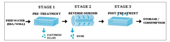
Figure 6: The three stages of the desalination process in a Reverse Osmosis plant.
