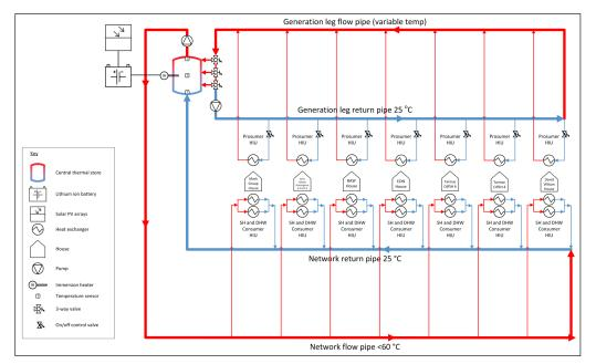
Figure 2: SCENIC double loop heat network with system components. Generation loop (top) facilitates heat transfer from distributed sources to CTS. Network loop (bottom) facilitates heat supply to houses from CTS.
