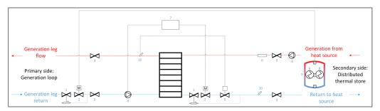
**Figure 6:** Danfoss FlatStation – 3 Series BS Basic Fully Insulated Indirect Prosumer HIU circuit diagram. Key: 1 – differential pressure controller, 2 – on/off valve, 3 – isolation valve, 4 – pump, 5 – thermostatic valve, 6 – energy meter, 7 – electrical wiring box, 8 – heat exchanger, 9 – hot water tank with immersion temperature sensors, 10 – temperature sensor node.
