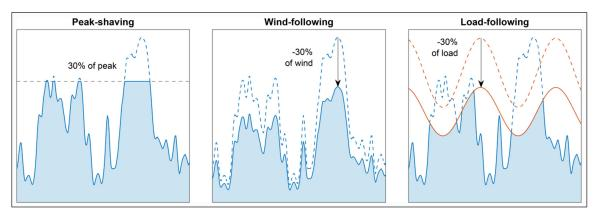
**Figure 1:** Schematic illustration of the different wind power curtailment methods using a curtailment rate of 30% as an example.
