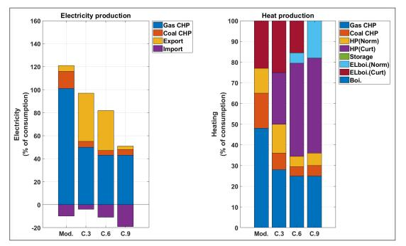
**Figure 6:** Electricity production and heat production of the power plants with different building energy savings, 1500 MW of heat pumps, wind curtailment, and dynamic heat pump COP for Scenario 4 (cases 6 and 9 in Table 7). The base system is here a modification of the present system.
