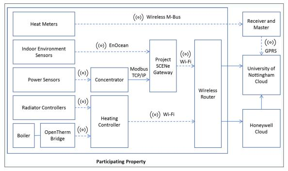
**Figure 3:** Architecture of the in-home monitoring equipment and cloud connections. Data leaves the property over the public Internet via the router's broadband connection or wirelessly for the heat meters. Dashed lines show wireless connections and solid lines physical connections.
