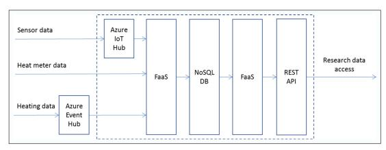
**Figure 4:** Key elements of the cloud service architecture. Services shown within the dotted area are part of the University of Nottingham's cloud infrastructure hosted on Microsoft Azure. The heating data Event Hub is part of the Honeywell cloud infrastructure, which is also hosted on Microsoft Azure. Data is stored and retrieved as documents using server-less functions or Functions as a Service (FaaS).
