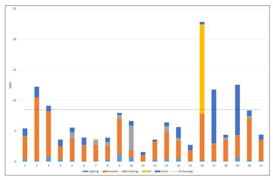
Figure 6: Disaggregated electricity consumption for each of the 21 sample properties over the same 24-hour period.
