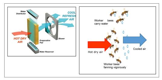
**Figure 6: (a)** Evaporative (swamp) cooler working principle. Image taken from (Richmueller, 2012); **(b)** an illustration of evaporative cooling performed by the worker bees.
